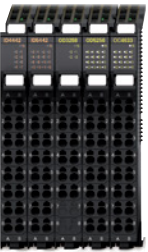
Digital I/O · 4, 8, 16, or 32 channels per input unit · 2, 4, 8, 16, or 32 channels per output unit (8 channels per relay output unit) · 16 channels per mixed I/O unit · Standard, high-speed, and time-stamp models · Units with Push-In Plus/MIL/Fujitsu/M3 Screw connector
